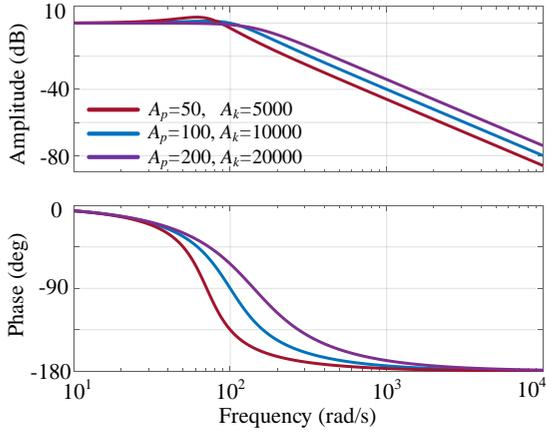
Fig. 10. The Bode plot of the IPLLL under different bandwidths.
