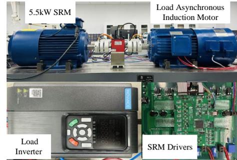
Fig. 14. Three-phase 12/8 SRM experimental setup.
