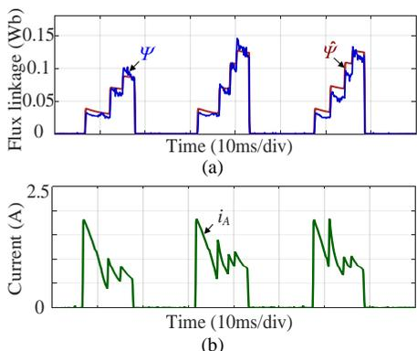
Fig. 15. Experimental results of flux linkage and current at 300r/min. (a) Comparison between calculated flux linkage  $\Psi$  and lookup table flux linkage  $\hat{\Psi}$ . (b) Phase current.
