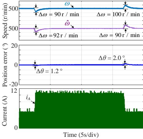
Fig. 20. Position-sensorless control under load change when loading to the rated current at 500 r/min.
