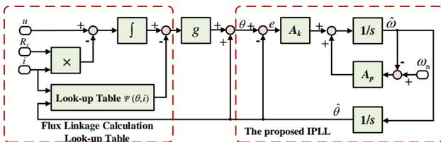
Fig. 13. Block diagram of the IPLL for the SRM sensorless control.
