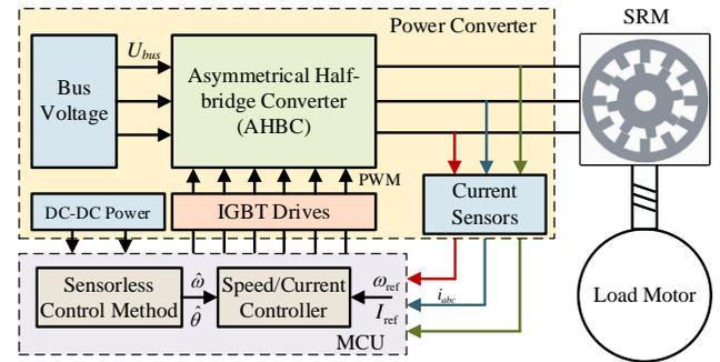
Fig. 1. The control diagram of the three-phase 12/8 SRM sensorless drive.
