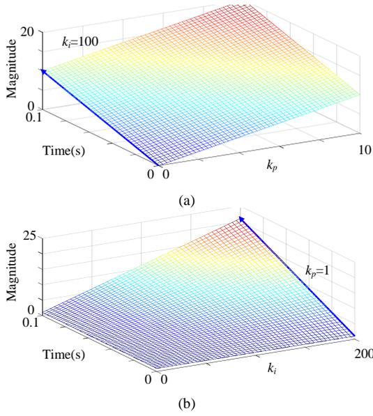
Fig. 6. The unit-step responses of the conventional PLL with various control parameters. (a)  $k_i=100$ . (b)  $k_p=1$ .
