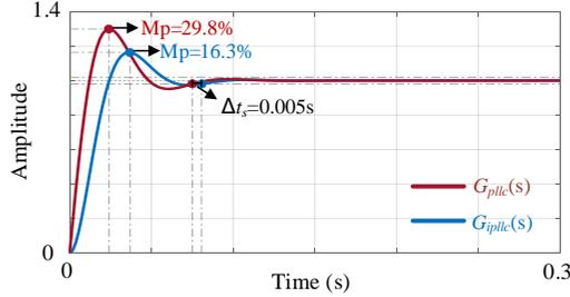
Fig. 12. Comparison of unit step responses between IPLL and proposed PLL with the same parameters.
