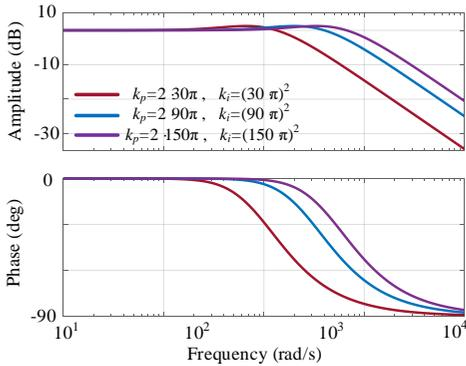
Fig. 7. The Bode plot of the conventional PLL under different bandwidths.
