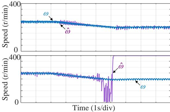
Fig. 21. Comparison of the proposed sensorless scheme and the conventional PLL scheme in the deceleration experiment from 250 r/min to 200 r/min.
