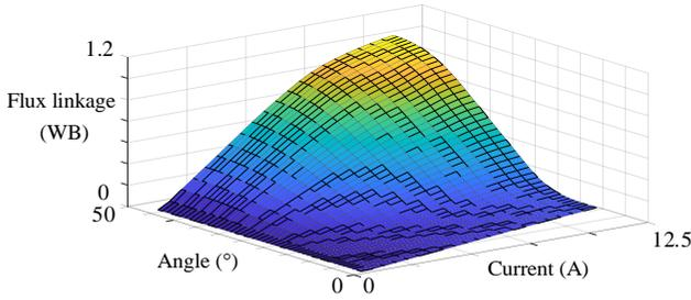
Fig. 3. Flux linkage profile of the studied SRM.
