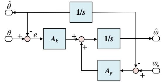
Fig. 8. The block diagram of the proposed IPLL.
