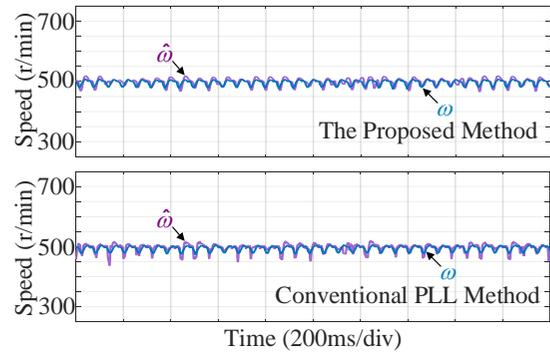
Fig. 19. The comparison experiment of steady-state speed tracking performance at 500 r/min.
