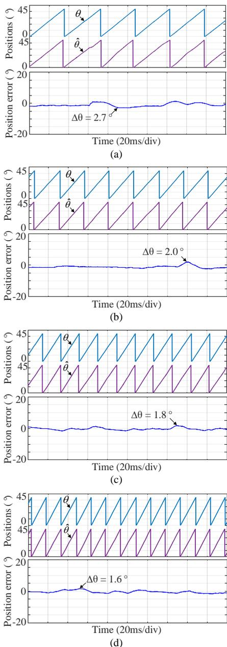
Fig. 16. Position estimation results of the proposed sensorless method. (a) 200 r/min. (b) 300 r/min. (c) 400 r/min. (d) 500 r/min.
