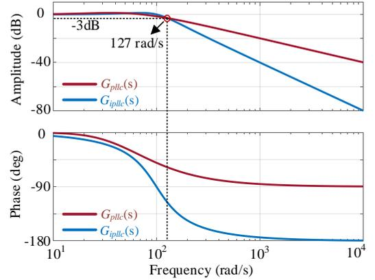
Fig. 11. Comparison of Bode plots for PLL and proposed IPLLL with the same bandwidth.
