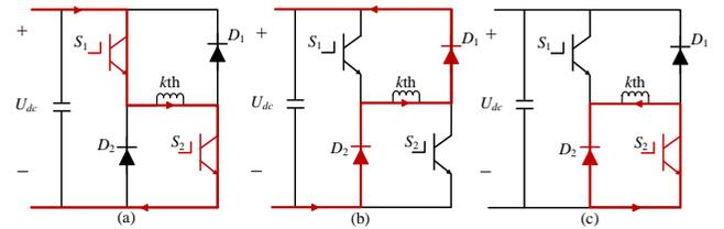
Fig. 2. Switching operating modes of the asymmetrical half-bridge converter. (a) Magnetization. (b) Demagnetization. (c) Freewheeling.
