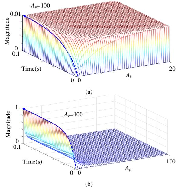
Fig. 9. The unit-step responses of the proposed IPLL with various control parameters. (a)  $A_p = 100$ . (b)  $A_k = 100$ .
