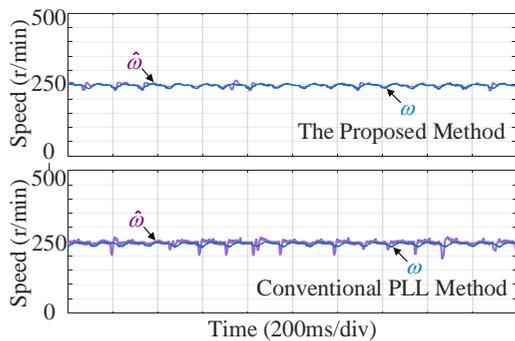
Fig. 18. The comparison experiment of steady-state speed tracking performance at 250 r/min.
