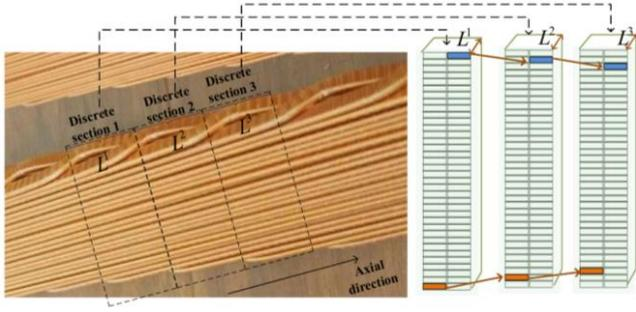
Fig. 9. Schematic diagram of discrete sections of parallel-wound transposition strands of stator windings [35].
