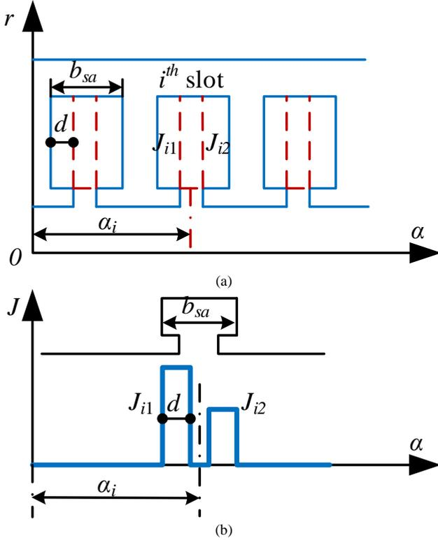
Fig. 4. Two-circumferential-layer winding. (a) Alternative winding layouts. (b) Current density function [12].
