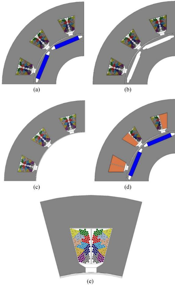
Fig. 6. Comparison of models for simplification [23]. (a) Quarter model. (b) No permanent magnet model. (c) No rotor model. (d) Single coil strand modeling model only. (e) Single slot model.
