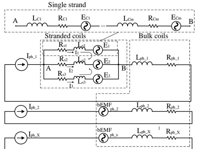
Fig. 5. Equivalent circuit structure [18].
