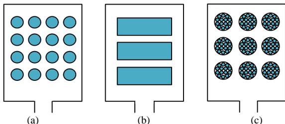
Fig. 10. Wire type. (a) Stranded Winding. (b) Flat Wire Winding. (c) Litz Wire Winding.
