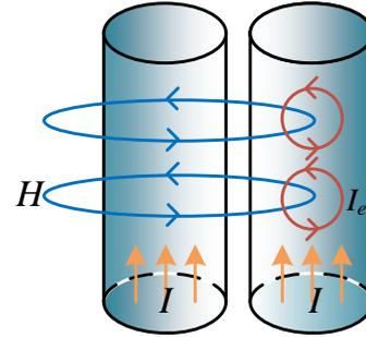
Fig. 2. Schematic diagram of proximity effect.
