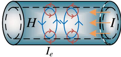
Fig. 1. Schematic diagram of skin effect.
