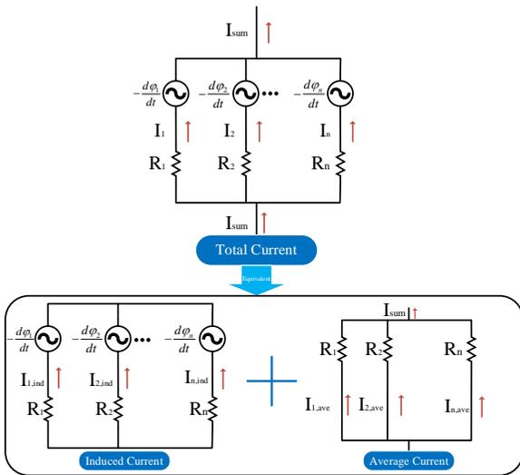
Fig. 8. Circuit model with n parallel strands [34].
